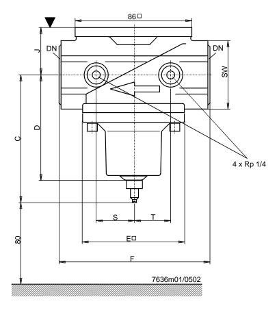
▼ Mounting surface for actuator or AGA60 adapter flange for SAX31... actuator
