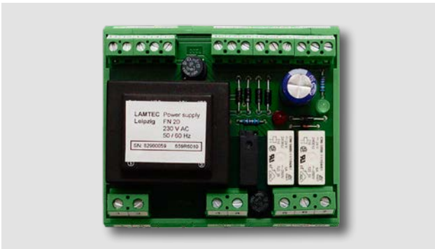
FN20 for top hat rail assembly FN20 in the connection housing with FSB connector, not shown.
