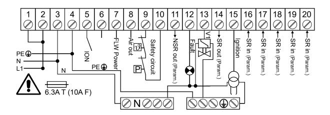
\* The connection lines used must be suitable for an ambient temperature of at least 75 °C (167 °F).
