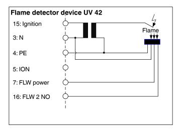
Use ignition lines with internal resistance (e.g. carbon fibre) or, in the case of ignition lines with a copper core, use ignition plugs with integrated interference suppression of at least 1 k $\Omega$ .
