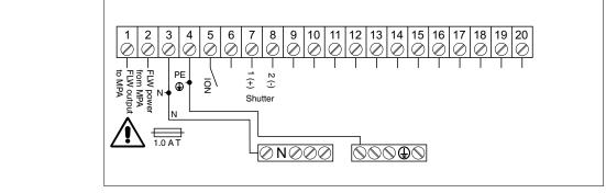
The flame detector device is also supplied with 230 VAC in the 115 VAC version via "Supply Flame Detector", terminal 7.
