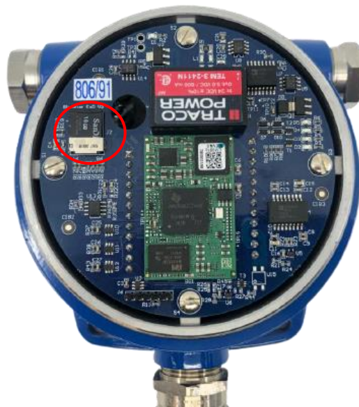
Figure 10: BlueEye™ Ex-D PCB with microSD card
